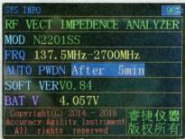
In Single Frequency mode or Scan Function interface, hold down the CTRL key (left), then press the M key, you can switch to the System Information interface.
