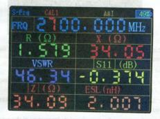
This interface is used for measuring the fixed frequency point.
