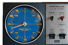
Type of installation: inside the rotor-controller
