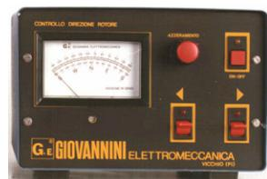
**ATTENTION:** as the rotator needs very high current you have to use the HEAVY-DUTY-version (1x ON/OFF 8A) of the ERC.
