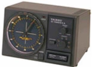
Type of installation: externally via a 6-pole Mini-DIN-Connector.
